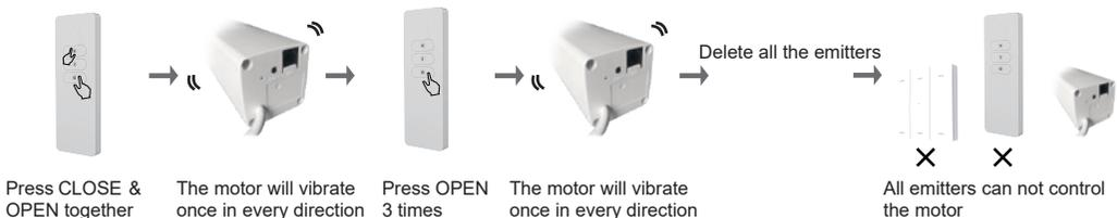
**Factory reset** After factory reset, the motor will lose all positions. At this time, the first manual function will be the first choice .
